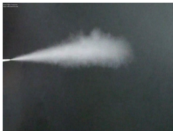
Fig. 7. High-speed photograph of optimal powder exit from the device loaded with 10 mg powder.
